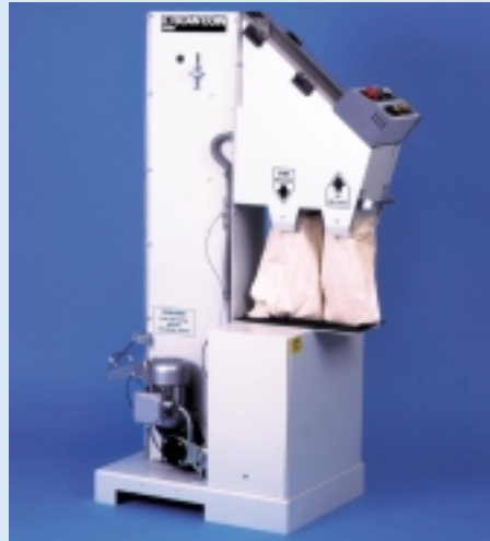
Vertical Cloth Bagging Station
