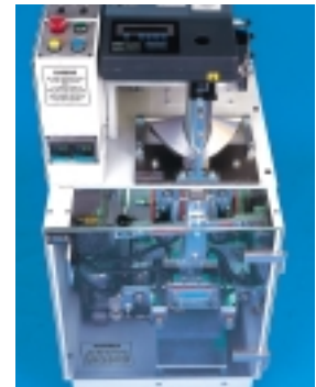
Temperature controls ensure sachets are correctly sealed
